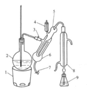
Figure A.1: Diagram of Nitrogen Distillation Device
